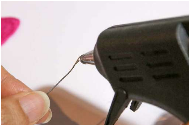
Step 2 - Start with the metal wire, apply a drop of hot glue to its tip
