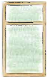
Reveal overlay doors and drawers partially overlap the face frame.
