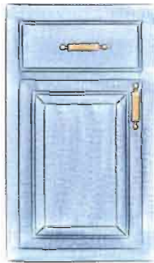
A drawer with beaded edge over a frame-and-raised-panel door, inset in face-frame case
