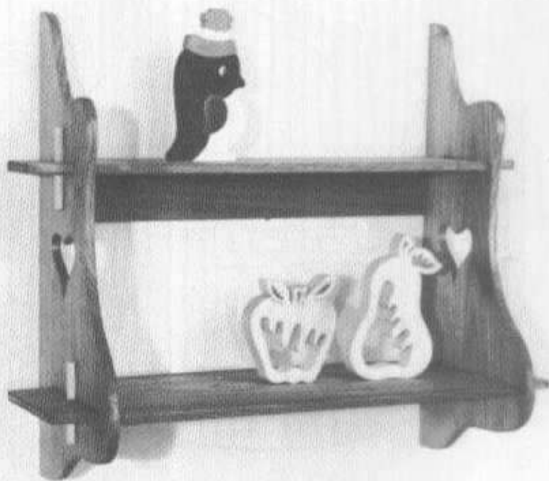
Wall shelf made of \frac{1}{4} " thick wormy butternut.
