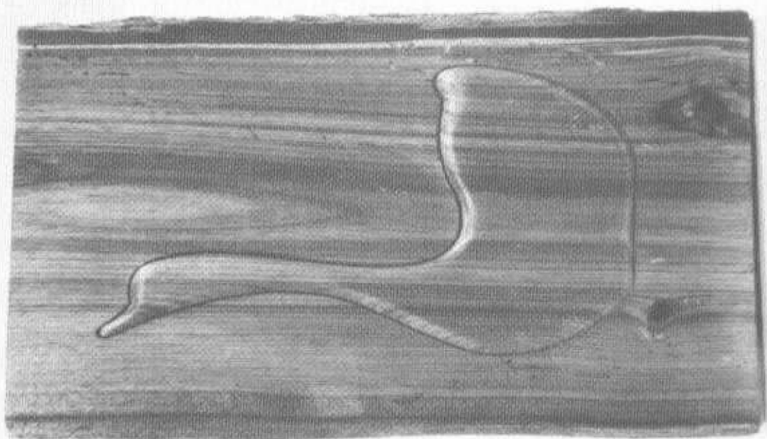
Rear view, showing the bead of hot glue applied around the relief inlay.
