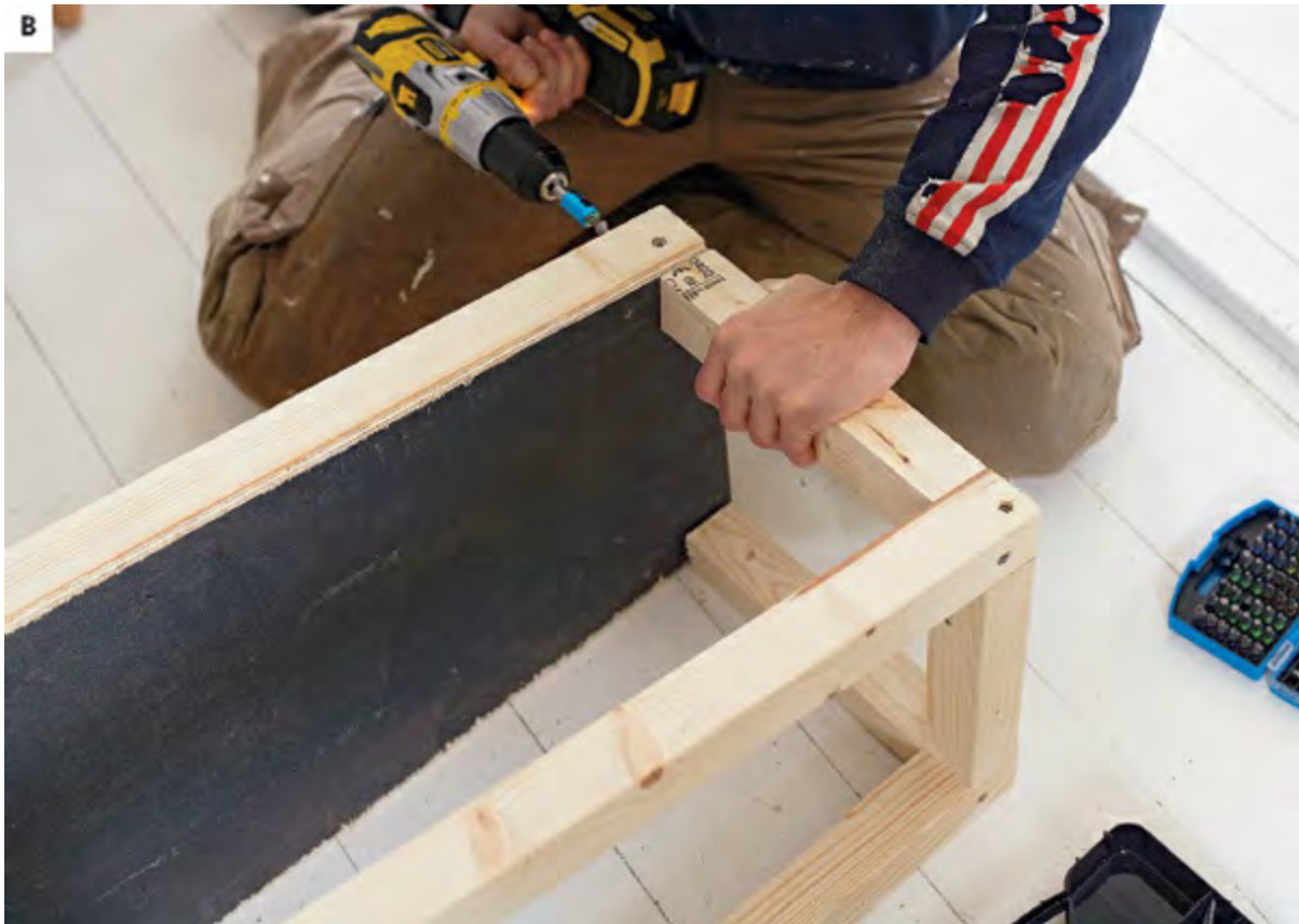
A–B. Start by assembling the undercarriage. Attach the board (which will become the floor of the car) to the undercarriage. Then put together the rest of the frame.
