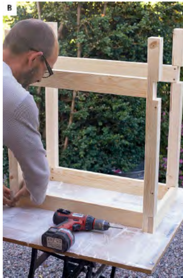
B. Assemble the entire leg construction with screws.
