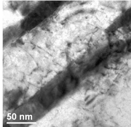
**Fig. 4.** Dislocation lines tangled at nano-wires in a sample prior to annealing. Two samples are marked by arrows. No. 1 shows a straight section between the wires and No. 2 is bent around a wire
