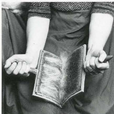
18 Transfer the wool from one card to the other. Note the position of the hands: cards upward, palms upward.
