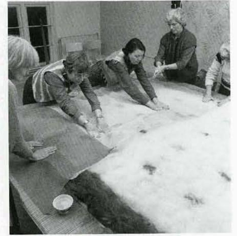
**80** The blanket was covered with screening, sprinkled with soapy water, and the air pressed out. Then it was rubbed.
