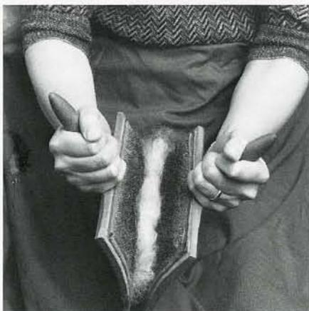
19 Making a small roll, a rolag. The hands are pulled upward, alternately, with short jerking motions. The wool forms a roll.
