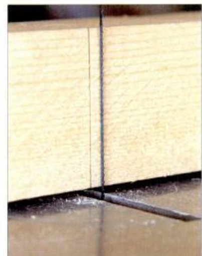
1–5. Test the fit of the blade in the kerf to see if your scrollsaw's table is square.
