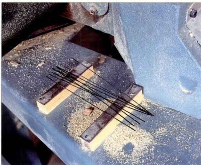
1–6. Make this handy scroll saw blade holder from magnetic strips and scrapwood.
