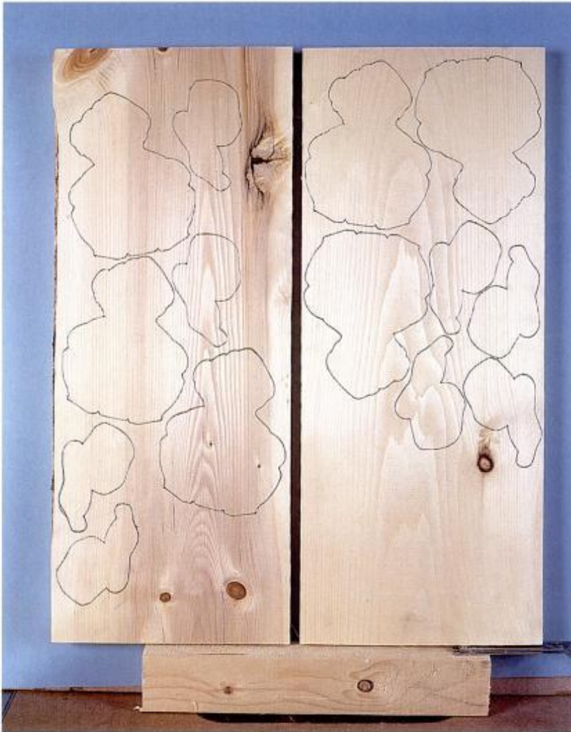
1–3. Pine is a good softwood to use for scrollsawing. On the left is No. 3 pine. On the right is No. 2 pine. No. 3 pine is less expensive, but has more knots. However, you can work around these defects to utilize most of the board.
