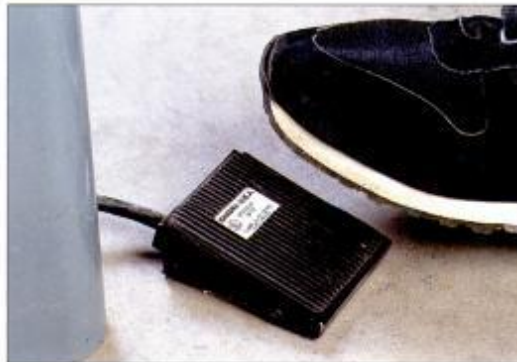
1-12. A foot-operated on/off switch will prove to be a helpful accessory because it allows the operator to use both hands to control the workpiece.
