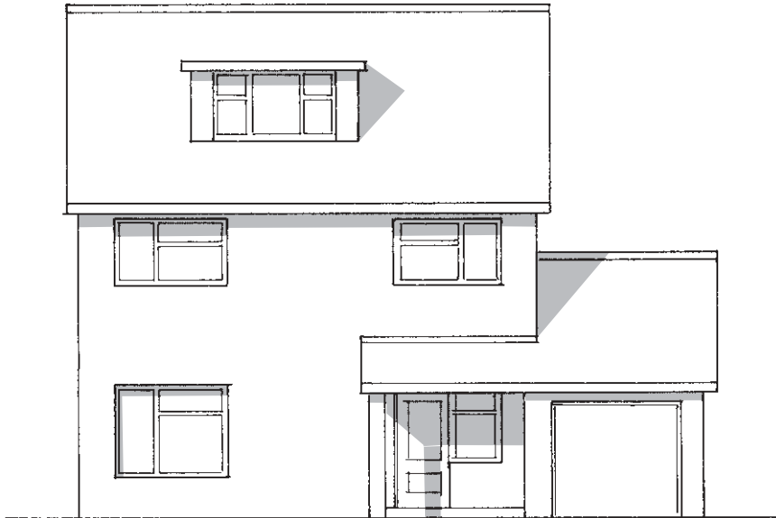
Fig.10.1 Poor dormer design.
