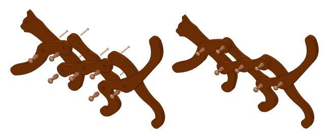
2. Fasten the Supports (part 9) onto the backs subassembly from the previous step with Woodscrews D4 x 20mm (part 10).
